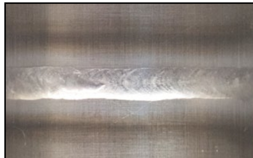
Acceptable weld made in AL-6XN mechanically polished tubing
