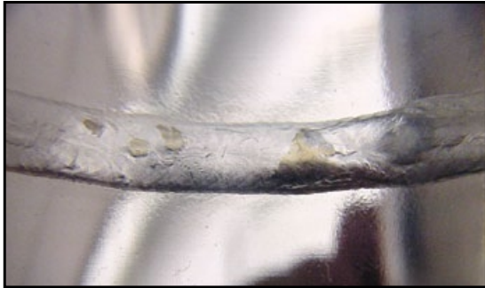
Acceptable weld made in AL-6XN electropolished tubing
