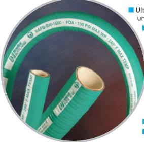
Ultra smooth, white, chlorobutyl rubber liner offers high purity and allows unrestricted flow; minimizing entrapment and blockage concerns
